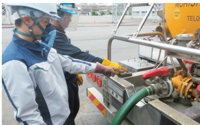
Receiving chromium effluent at the Tokuyama Factory
